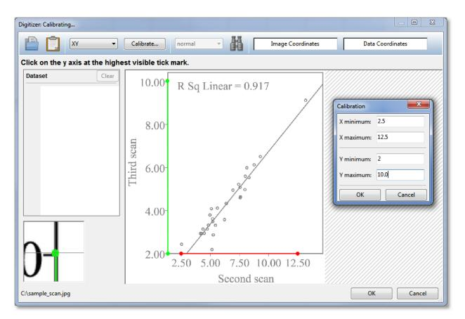
Remember that you can still fine-tune the location of the calibration points by pointing at them with the mouse and using the arrow keys to move the calibration point to the desired location. Any data points that you have already created will be automatically adjusted as the calibration changes.
