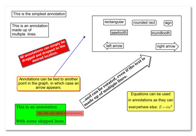
To add a new annotation, press the Annotation button in the *Graph Toolbar*, or press the N key while in a graph. When adding an annotation, the annotation properties dialog will appear, which is documented below. Another way to create an annotation is to clone an already existing one, by right clicking an annotation and picking **Clone** from the resulting menu.
