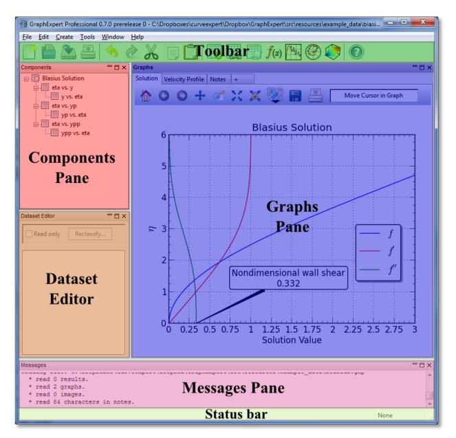
All of the panes can be shown or hidden via the *Window* menu in the menu bar. Further, panes (except for the Graphs pane) can be torn out from the main window; grab the pane by its title bar, and tear it out. The panes can be redocked in the main window by the reverse operation; drag the window to one of the docking indicators, and a transparent hint will appear to show where the window will be docked. Using this procedure, the panes can be rearranged inside the main window to taste.
