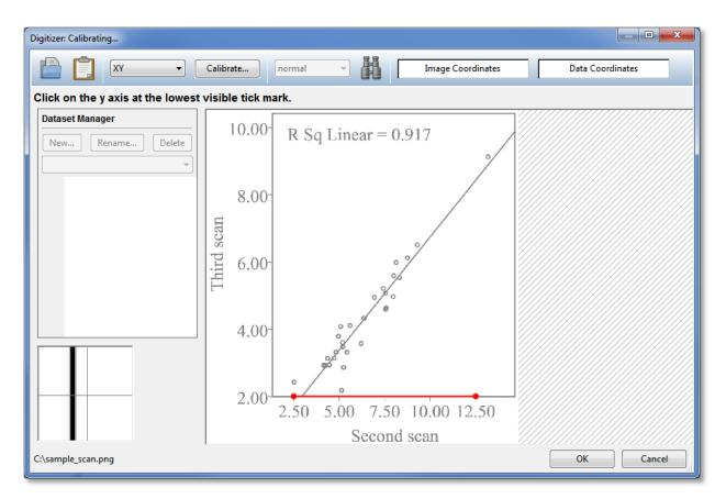
After specifying the X axis calibration, we will now specify the calibration for the Y axis. In the same manner as the X axis was calibrated, click on the Y axis at the lowest possible tick mark on the Y axis, and then at the highest possible tick mark on the Y axis. The Y axis calibration points will be indicated by green points connected with a green line.
